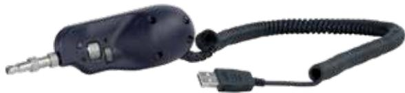
Make sure to have clean connector installed. A dirty connector will increase the power loss! Inspect your connector before and after cleaning.
